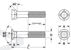
‡Length of a plow bolt is measured from the top of the head to the extreme end of the bolt.
