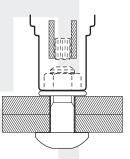
When the proper bolt tension is reached, the tip of the bolt will shear. When the tip of the bolt shears, pull back on the wrench until the outer socket is no longer engaging the nut.
