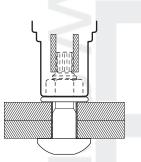
Slide the inner socket over the bolt tip and the outer socket over the nut. Press the trigger switch. The outer socket will rotate and tighten the nut until the bolt reaches the required tension.
