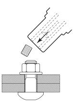
Push the ejector lever to discharge the severed bolt tip.
